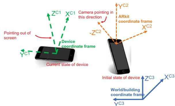
Figure 2: Different coordinate frames: C1 (device), C2 (AR), C3 (world)
