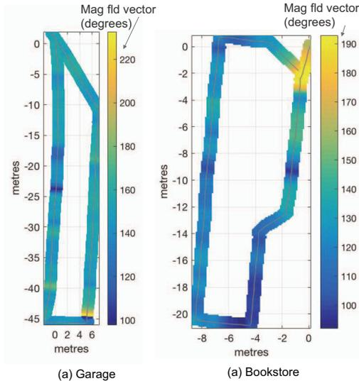
**Figure 3: Magnetic field map of real world environments**
